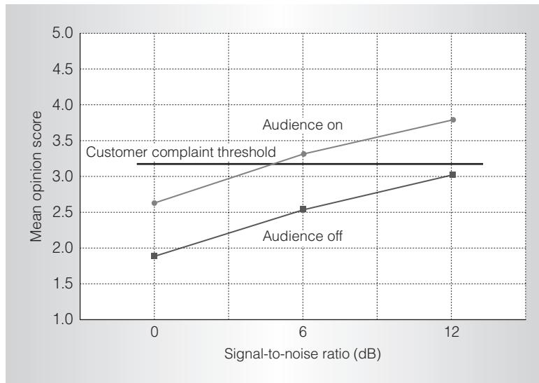
Figure 9. Subjective performance measurement using ITU-T P.835 Amendment 1, Appendix III methodology. The Audience A1010 voice processor improves performance an average of 0.77 MOS.
