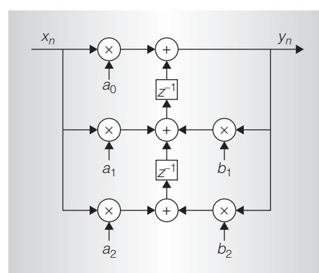
Figure 4. Biquad filter used in Lyon's cochlea model, in which  $y_n = a_0x_n + a_1x_{n-1} + a_2x_{n-2} + b_1y_{n-1} + b_2y_{n-2}$ . The Audience A1010 voice processor uses a proprietary variation of this method.
