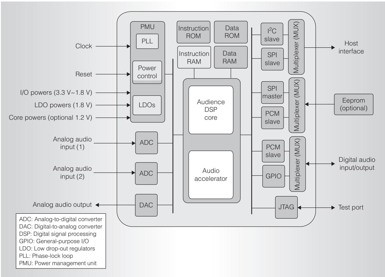
Figure 6. Block diagram of Audience's A1010 voice processor chip. The power management unit includes the clock phase-lock loop and low drop-out regulators. Analog-to-digital and digital-to-analog converters provide the analog interfaces. The voice processor supports several industry standard interfaces, including I<sup>2</sup>C (inter-IC communication), SPI (serial peripheral interface), PCM (pulse-code modulation), and GPIO (general-purpose I/O).
