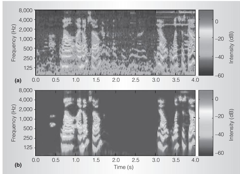
Figure 8. The fast cochlea transform (FCT) representation of a microphone signal before (a) and after (b) noise reduction. The logarithmic frequency scale shows a doubling in frequency (each tic mark represents doubling). The signal is a voice recorded on a busy street with traffic noise, a nearby talker, and a cell phone ringtone.
