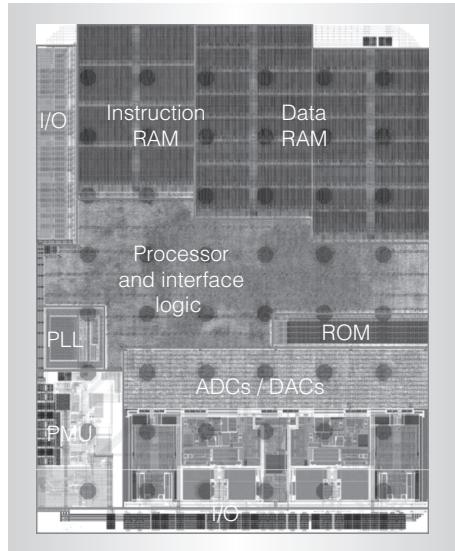
Figure 7. Die plot of the A1010 voice processor. Memory (RAM and ROM) occupies about a third of the area; mixed-signal functions (analog-to-digital and digital-to-analog converters) occupy about a third of the area; and processor logic and power management functions occupy the rest of the area.
