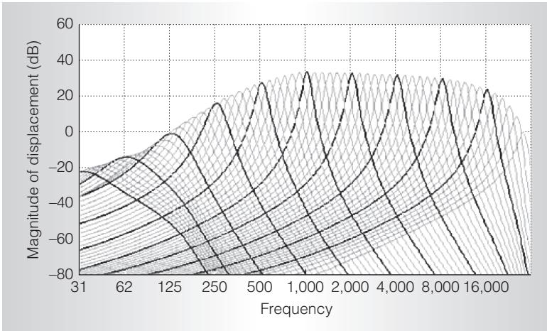
Figure 5. Transfer functions of the cochlea model. These filter responses were carefully designed to match the bandwidths and peak amplitudes of the human hearing responses.
