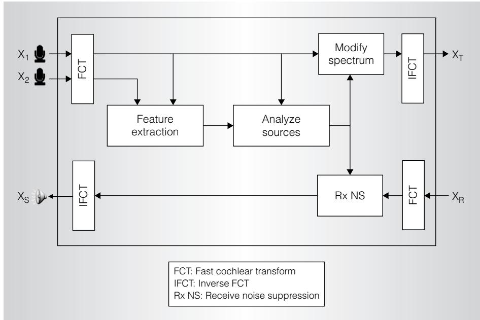
Figure 3. Block diagram of the computations performed in the Audience voice processor. The transmit noise reduction functions flow from left to right; the receive noise reduction functions flow from right to left.
