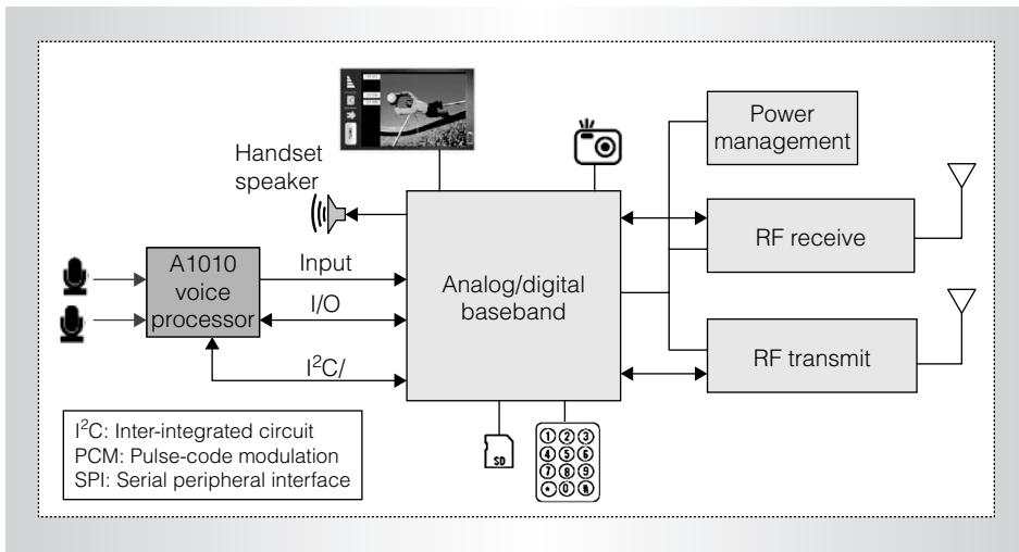
Figure 1. Mobile phone architecture. The Audience A1010 voice processor resides between the microphones and baseband processor, providing advanced noise reduction.
