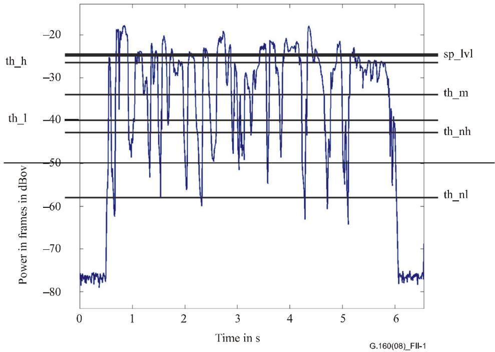
**Figure II.1 – Power in frames of clean speech as a function of time
