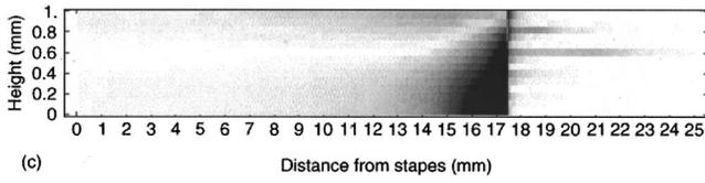
FIG. 3. Relative Laplace error (RLE) shown as a density plot as a function of position in the duct, for Neely's parameters with  $f=2.26$  kHz. White corresponds to  $RLE=0$ ; black corresponds to  $RLE>1$ .
